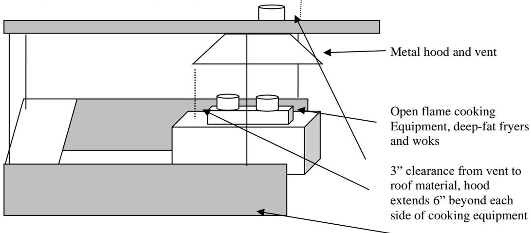
A booth can be made of fire retardant treated combustible material e.g., wood, fabric, etc. provided it:
