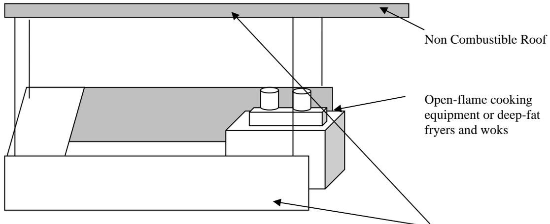
If the booth siding and top are made of noncombustible materials i.e., metal, cement board, sheetrock, etc. then open-flame, deep-fat frying or wok type equipment may be used inside booth. Booth framework may be constructed of wood.
